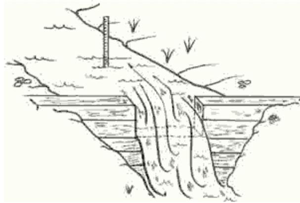
It's important to note that your depth measurement is not taken at the gate itself because the water depth distorts as it moves through the gate. Instead, insert a stake well upstream of the Weir gate and make the top of the stake exactly level with the bottom of the Wier gate. Measure the depth of the water from the top of the stake.
