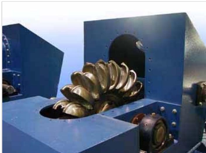
*Pelton-type impulse turbine with housing cover removed.*
