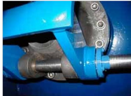
*Close-up of jet deflector in position to deflect the water jet away from the turbine.*
