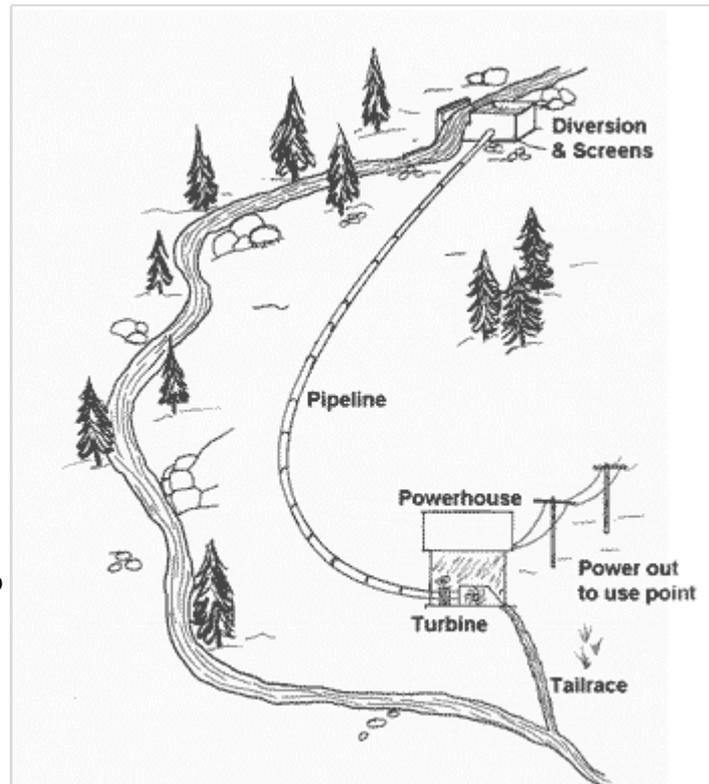
*Major components of a hydro system include a water diversion, pipeline to create pressure, turbine & generator, tailrace for exiting water, and transmission wires.*
